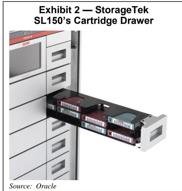
acquisition hit. The StorageTek SL150 base unit (shown at the top of the cabinet in Exhibit 1, on the previous page) has a four-cartridge mail slot for the import and export of LTO media. Each drawer type, both base and expansion, supports two half-height LTO-5 drives at 6Gbps using FC or 8Gbps with SAS, for a maximum throughput of 10TB/hour. (See cartridge drawer photo in Exhibit 2, to the right.) That equates to 450TB and 20 drives in only 21 rack units of height.
