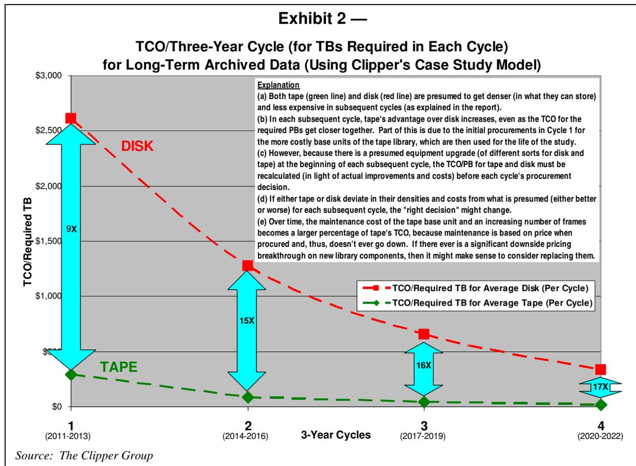
by the vendors. Our disk comparison point began with 2TB disk assembled into fully-configured arrays, which can be considered Tier-2 storage. Our tape comparison point began with *Ultrium* generation-5 (LTO-5)<sup>3</sup> tape cartridges and drives and housed in a fully-configured, enterprise-class *Automated Tape Library (ATL)*. Because we found that the cost of disk is about 15 times that of tape, we fully expect to see more discounting on the disk acquisitions than for tape<sup>4</sup>.
