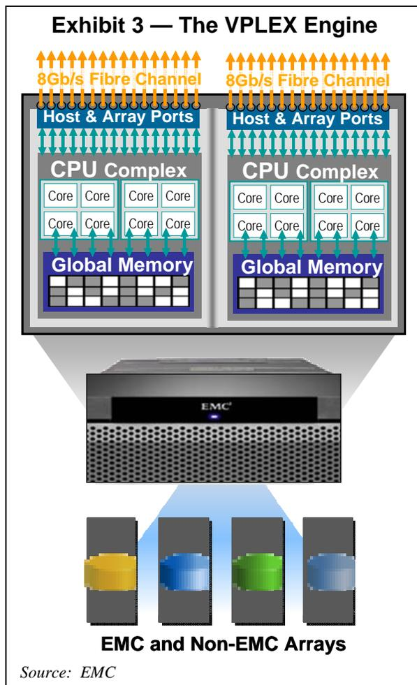
and the engine controlling the latest data needs only to share what has changed with the requesting engine, the volume of data to be transported has been reduced significantly, especially in comparison with a full transfer of updated block(s)
